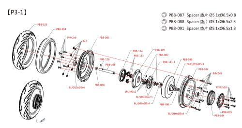
Note: Please coated the screw glue first when screwing down the flat head screw(M2x6).
