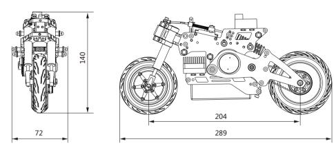
$Length: 289mm \\ Width: 72mm \\ Height: 140mm \\ Wheelbase: 204mm$
