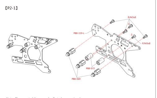
Note : Please coated the screw glue first when screwing down the flat head srew(M3x8) and the round head screw(M3x8). 提示: 锁平头螺丝 ( M3x8)和圆头螺丝(M3x8)时需先涂上螺丝胶。
