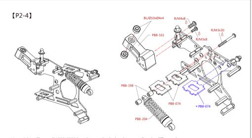
Note: Inject silicone oil #900-5000 into the rear shock absorber according the different site; Please coated the round head screw (M3x8) &(M3x30) &(M4x8).
