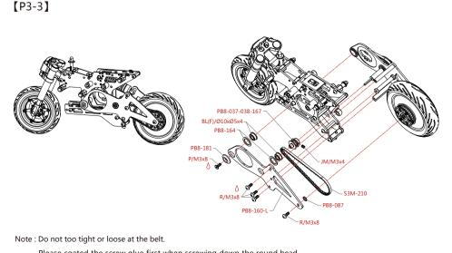
Please coated the screw glue first when screwing down the round head  $srcew(M3x8)\&The\ flat\ head\ screw(M3x8)\ and\ the\ grains(M3x4).$
