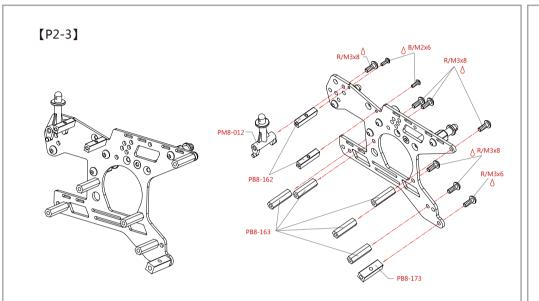
Note: Please coated the screw glue first when screwing down the round head screw (M3x8)&(M3x6)and the scoket head screw(M2x6). 提示:圆头螺丝 ( M3x8)&(M3x6)和杯头螺丝 ( M2x6)时需先涂上螺丝胶。
