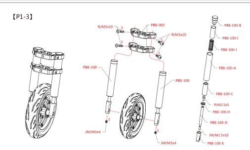
Note: Apply silicone oil #20000 on the spring, coated the screw glue first when screwing down the round head screw(M3x10) and the grains(M3x4). 提示:弹簧涂上#20000号避震油;锁圆头螺丝(M3x10)和机米(M3x4)时需先涂上螺丝胶。
